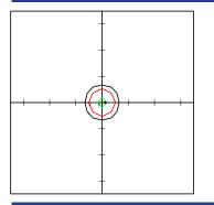
TAMLITE LIGHTING EMERGENCY AND FIRE ESLR-1 Horizontal Footcandles Scale: 1 Inch = 10 Ft. Light Loss Factor = 1.00 Lumens Per Lamp = N.A. Lumens = 45 Mounting Height =10.00 Ft Maximum Calculated Value = 0.69 Fc Arrangement: Single
