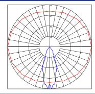
Polar Graph Maximum Candela = 76.5 Located at Horizontal Angle = 0 Vertical Angle = 2.5 Vertical Plane Through Horizontal Angles (0 - 180)Horizontal Cone Through Vertical Angle (2.5)
