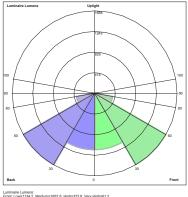
Luminaire Lumens: Front: Low=1134.2, Medium=1657.6, High=373.8, Very High=61.2 Back: Low=1134.2, Medium=1657.6, High=373.8, Very High=61.2 Uplight: Low=0.6, High=0.0 BUG Rating : B3-U1-G1
