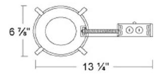
Housing adjusts to accommodate various ceiling thicknesses
