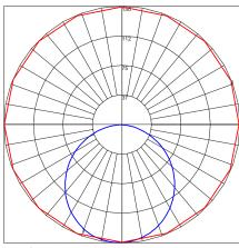
Maximum Candela = 149.84 Located At Horizontal Angle = 202.5, Vertical Angle = 3 # 1 - Vertical Plane Through Horizontal Angles (202.5 - 22.5) (Through Max. Cd.) # 2 - Horizontal Cone Through Vertical Angle (3) (Through Max. Cd.)
