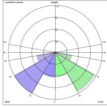
Luminaire Lumens: Front: Low=97.3, Medium=106.1, High=39.4, Very High=3.7 Back: Low=84.4, Medium=111.6, High=44.3, Very High=5.4 Uplight: Low=0.0, High=0.4 BUG Rating: B0-U1-G0
