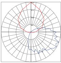
Maximum Candela = 3217.46 Located At Horizontal Angle = 90, Vertical Angle = 70 # 1 - Vertical Plane Through Horizontal Angles (90 - 270) (Through Max. Cd.) # 2 - Horizontal Cone Through Vertical Angle (70) (Through Max. Cd.)
