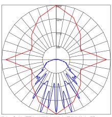
Maximum Candela = 2232 Located At Horizontal Angle = 90, Vertical Angle = 16.5 # 1 - Vertical Plane Through Horizontal Angles (90 - 270) (Through Max. Cd.) # 2 - Horizontal Cone Through Vertical Angle (16.5) (Through Max. Cd.)
