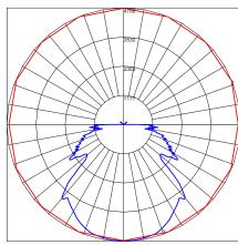
Maximum Candela = 4706 Located At Horizontal Angle = 67.5, Vertical Angle = .5 # 1 - Vertical Plane Through Horizontal Angles (67.5 - 247.5) (Through Max. Cd.) # 2 - Horizontal Cone Through Vertical Angle (.5) (Through Max. Cd.)
